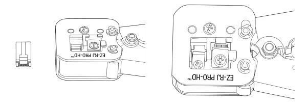
7. Once the tool is locked in the last ratchet position, use the screw driver to fully tighten blade with connector in place. This process aligns the blade properly for the next termination.
