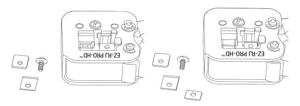
4. Place the new blade into tool ensuring the spacer is oriented correctly, the flat side of the blade is face down, and the angled side is showing.
