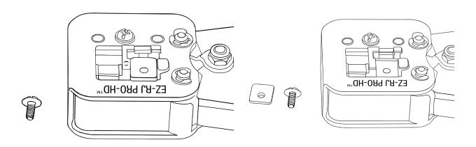
3. After removal of the front plate, remove the blade. Note the orientation of the blade. Once the blade has been removed, note the small spacer under the blade. This piece does not need to be removed to replace the blade. Although note that this piece has a specific orientation. The space from the screw hole is smaller on top than on the bottom.
