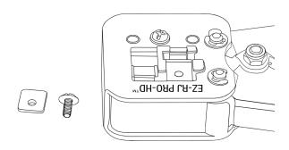
5. Orient the front plate with the flat side against the blade and all holes lining up. Insert screw and slightly tighten the screw with the screwdriver. The blade should still be loose.
