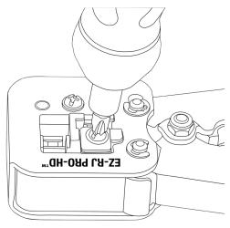
6. Once the screw has been tightened enough to leave the blade still loose, insert a crimped EZ-RJ45 Connector and cycle the tool down to the last ratchet point.
