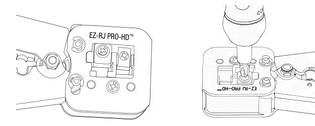
2. Once the screw has been removed, remove the front plate and set aside. Note: the front plate does have a front and a back side. The side pressed on the blade is flat and the screw side is rounded.
